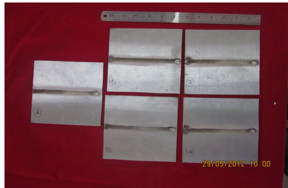
Fig. 2 Photographs of fabricated joints
