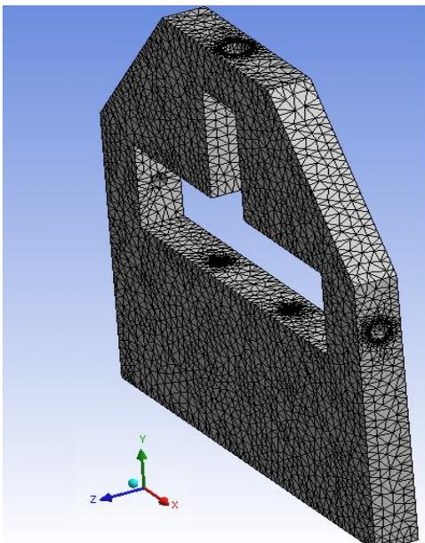
**Fig. 5 Meshing of the Frame**
