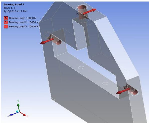
**Fig. 8 Applied Axial Bearing Load in Positive z Direction for Bottom Rollers and in Opposite Direction for the Top Roller**
