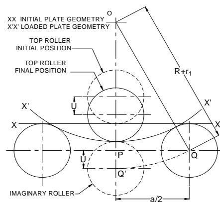
Fig. 1 Schematic Diagram of Three roller Bending Process
