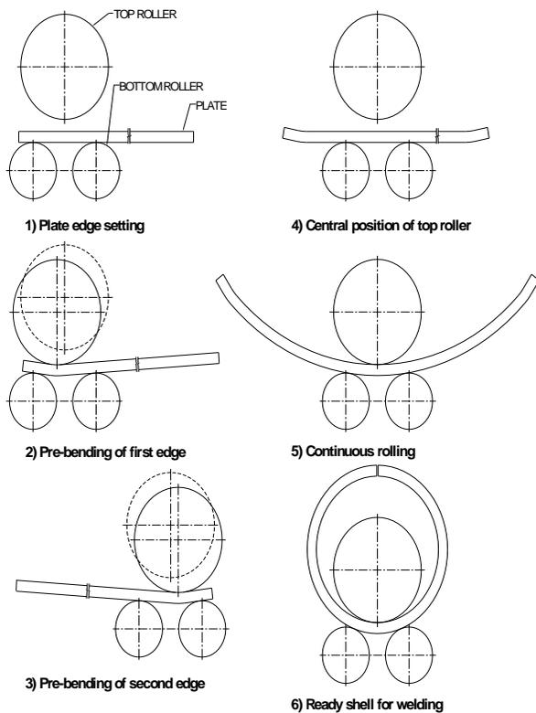
**Fig. 2 Roller Bending Sequence for Fixed Bottom Roller Gap**
