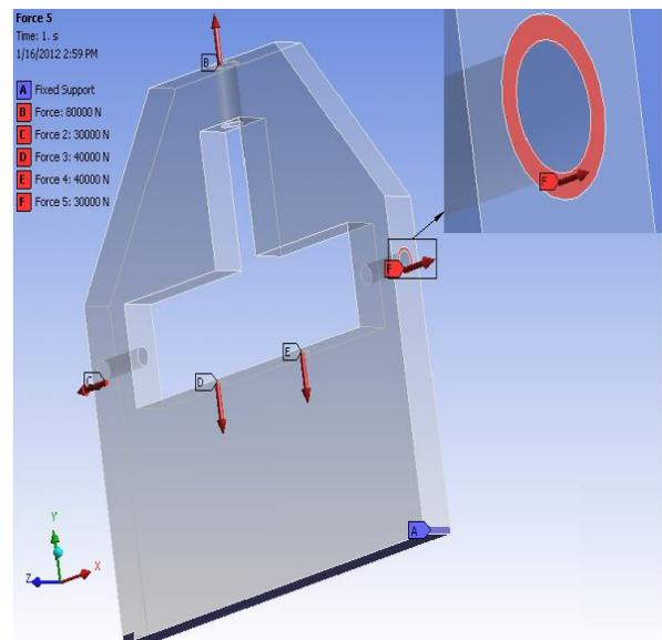
**Fig. 6 Applied Fixed Support and Forces in X & Y Directions**
