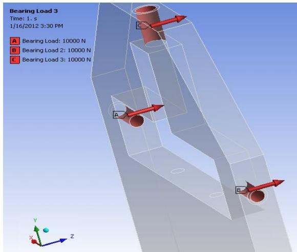
**Fig. 7 Applied Axial Bearing Load in Positive Z Directions for all the Tree Rollers**
