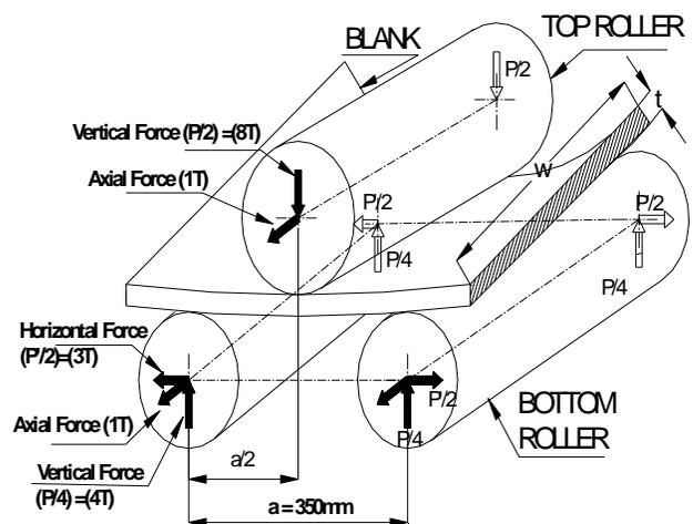
**Fig. 4 Forces on Rollers during Bending**
