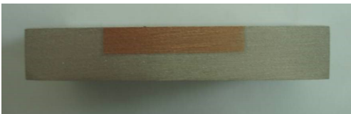
Fig. 2 Front view of welding sample section
