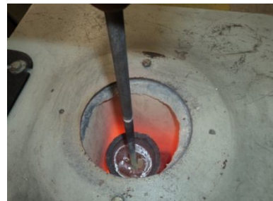
Fig. 1 Production of Al-SiC Composites
