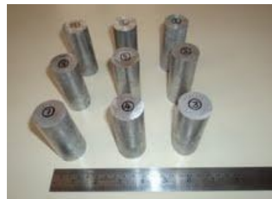
Fig. 2 Al-SiC Composite Specimens
