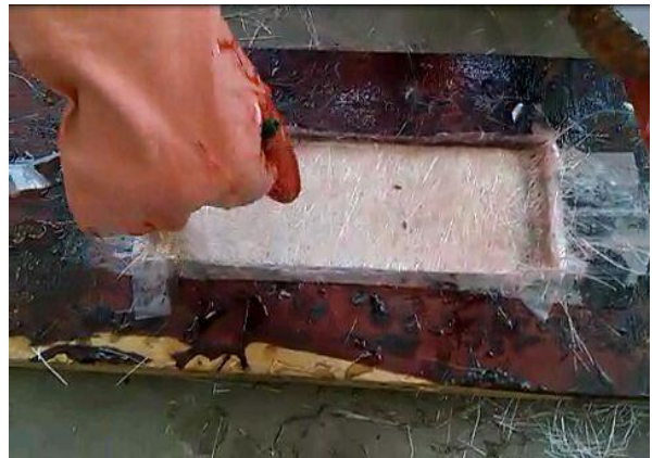
Fig. 2 Fabrication of GFRP Drilling Specimen
