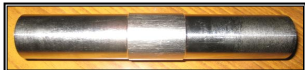
Fig. 4 Inconel 718 Bar (Machined)
