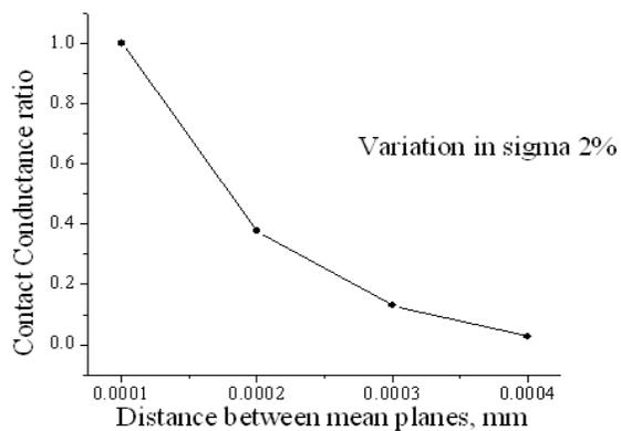
**Fig. 11** Variation in Contact Conductance for Roughness Set 2
