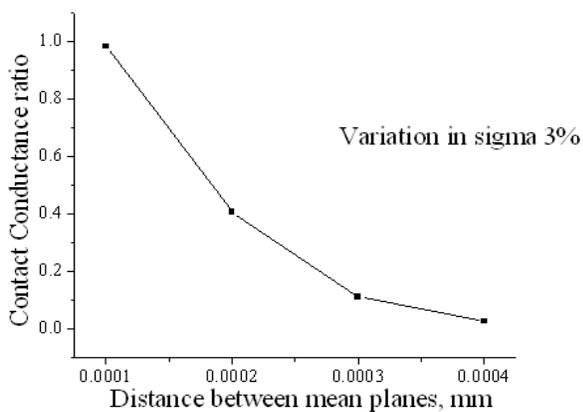
**Fig. 10** Variation in Contact Conductance for Roughness set 3
