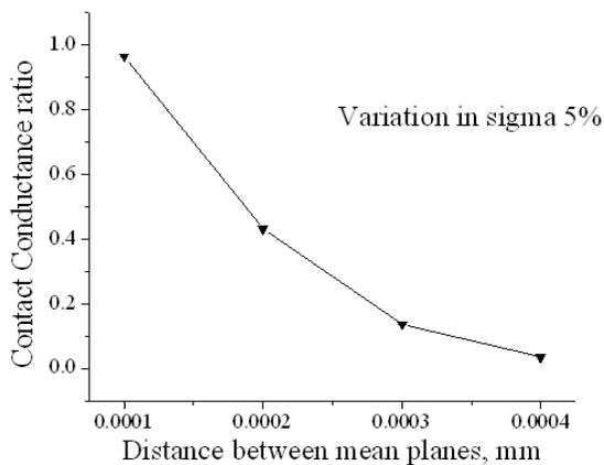
**Fig. 8** Variation in Contact Conductance for Roughness set 1
