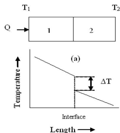
**Fig. 1 Temperature Drop due to Imperfect Joint**
