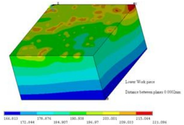
**Fig. 6 Temperature Distribution for Distance between Planes 0.0002 mm**
