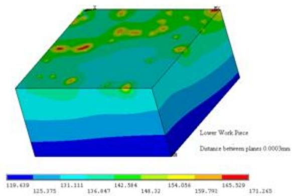
**Fig. 5 Temperature Distribution for Distance between Planes 0.0003 mm**
