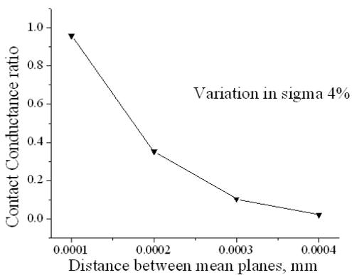
**Fig. 9** Variation in Contact Conductance for Roughness set 2
