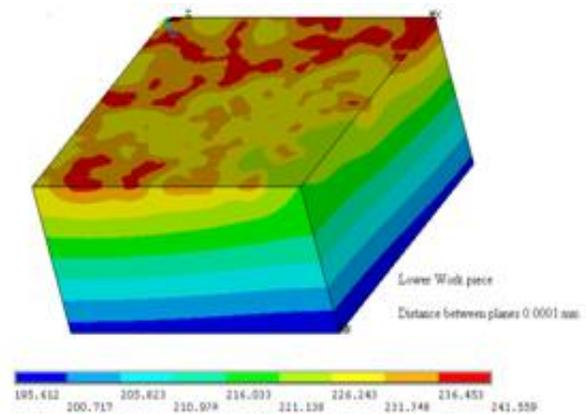
**Fig. 7 Temperature Distribution for Distance between Planes 0.0001 mm**
