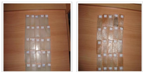
Fig.1 Photographs of the Specimens of PP and PMMA for Material Removal Test
