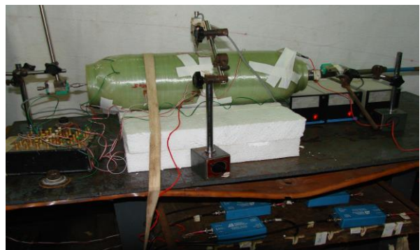
Fig. 3 Pressure Bottle Experimental Setup
