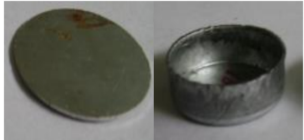
Fig. 5 A Sample of Blank and Cup Drawn
