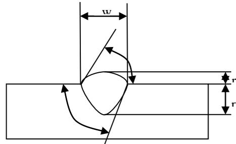
**Fig. 1 Elements of Bead Geometry**
