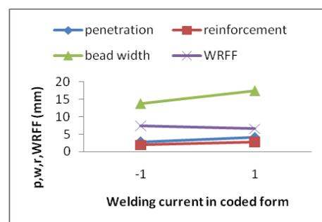
**Fig. 3 Effect of Welding Current on Bead Geometry**
