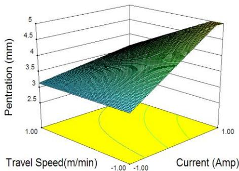
Fig. 6 Response Surface Due to Interactive Effect of Welding Current and Travel Speed on Penetration
