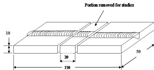
**Fig. 2 Specimen Cutting Plan**
