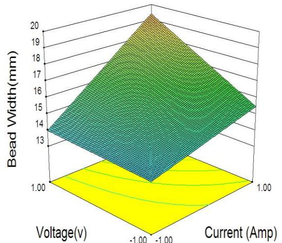
Fig. 8 Response Surface Due to Interactive Effect of Welding Current and Arc Voltage on Bead Width
