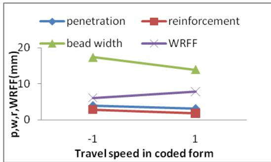
Fig. 4 Effect of Travel Speed on Bead Geometry
