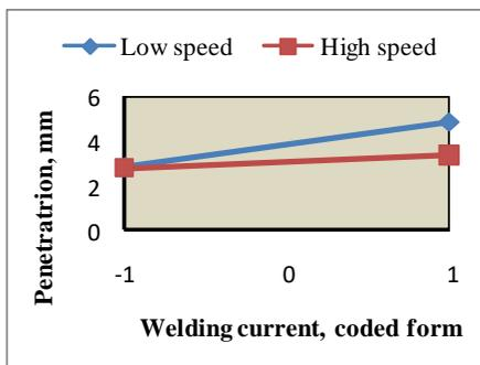
Fig. 5 Interactive Effect Welding Current and Travel Speed on Penetration
