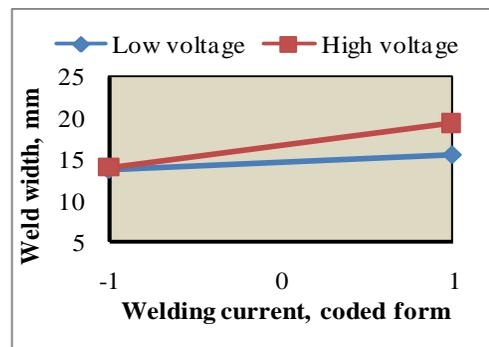
Fig. 7 Interactive Effect of Welding Current and Arc Voltage Weld Width
