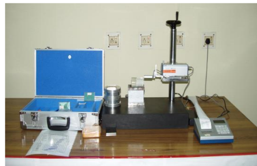
Fig. 2 Experimental Setup of Surface Roughness Tester
