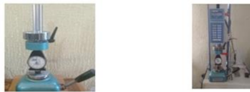
Fig. 8 (a) Shore D Hardness Tester, CV Instrument, England. (b) Shore D Hardness Tester installed on Tensile Machine
