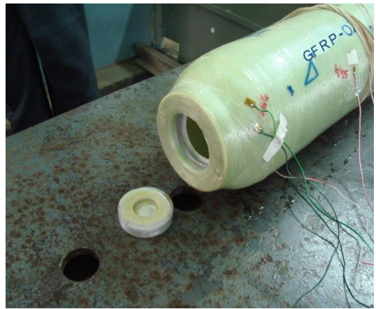
Fig. 5 Failure Mode of GFRP-02
