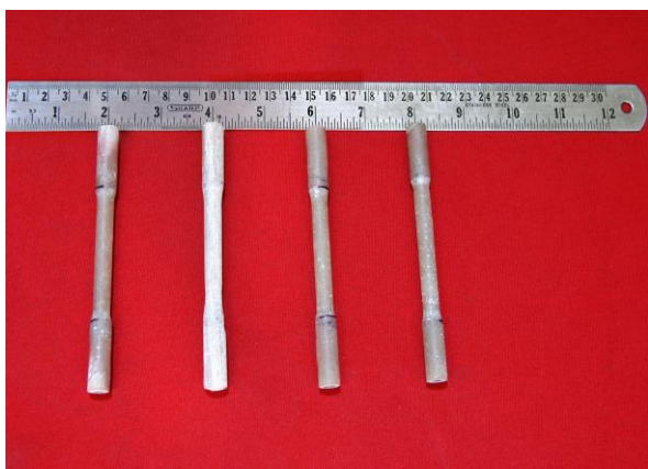
Fig. 1 Tensile Specimens before Testing
