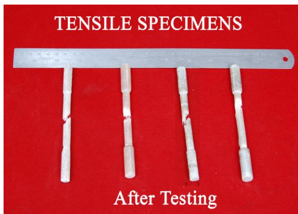
Fig. 2 Tensile Specimens after Testing
