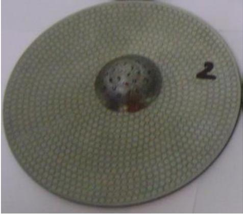
Fig. 16 Specimen after Erichsen Test
