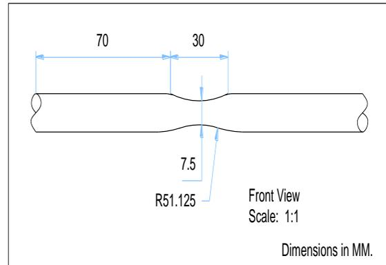
**Fig. 1 Specification of the Fatigue Test Specimen**
