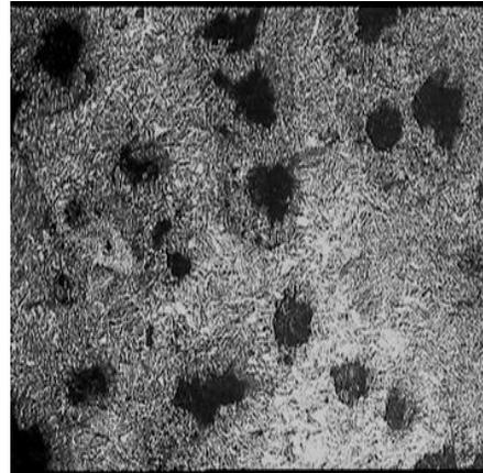
**Fig. 7 Representative Photomicrographs of TADI for Austempering Time 120 min**
