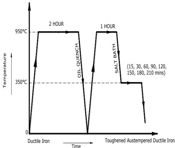
Fig. 2 Special Austempering Heat Treatment Cycle
