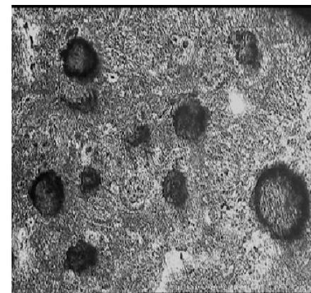
**Fig. 9 Representative Photomicrographs of TADI for Austempering Time 180 min**
