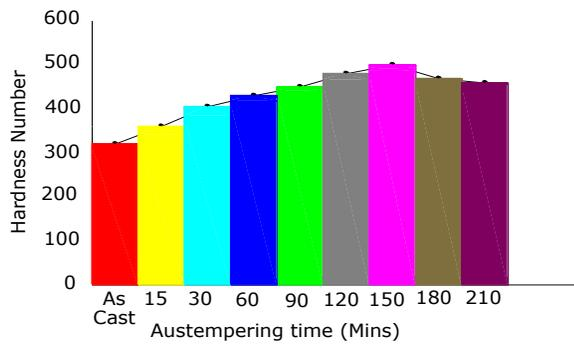
**Fig. 4 Variation of Micro Hardness Value with Austempering Time of TADI**
