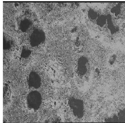
**Fig. 8 Representative Photomicrographs of TADI for Austempering Time 150 min**
