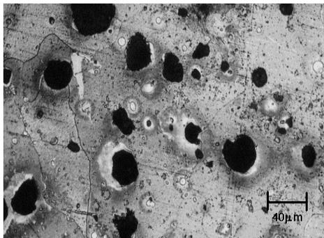
**Fig. 5 Photomicrograph of as Cast Ductile Iron**
