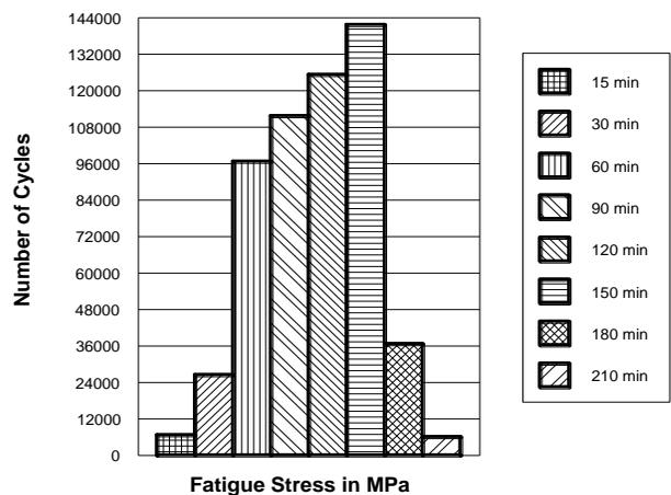
Fig. 3 Variation of Fatigue Value with Austempering Time of TADI
