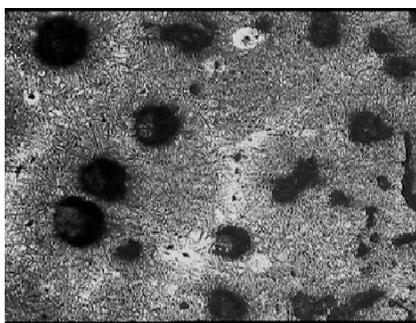
**Fig. 6 Representative Photomicrographs of TADI for Austempering Time 60 min**
