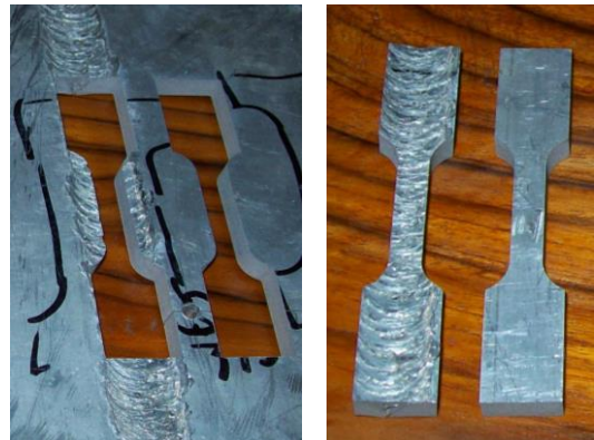
Fig. 6 Sample Drawing and Specimens Extracted for Tensile Test
