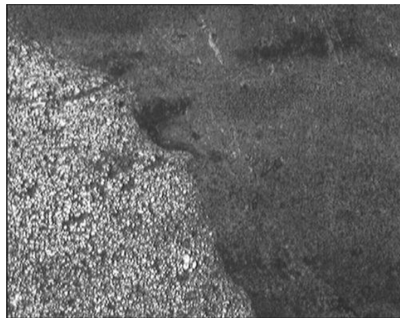
(e) Weld cross section showing the weld line
