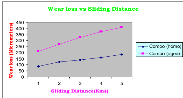
Fig. 5 Sliding Wear Behavior of Composite (Homogenized and Aged, T 6 )
