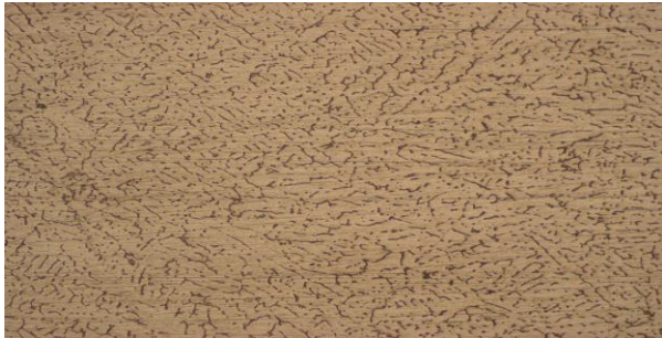
Fig. 1 (a) Optical Microstructure of Al-Cu Alloy (100X )
