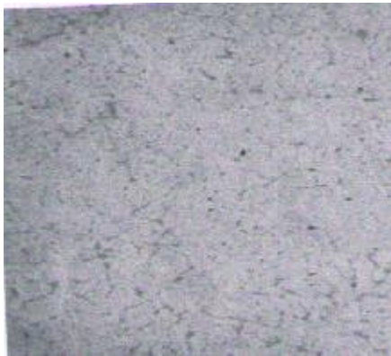
Fig. 2 Microstructure of Al 6061- Ni-Ce-0% (400 x)
