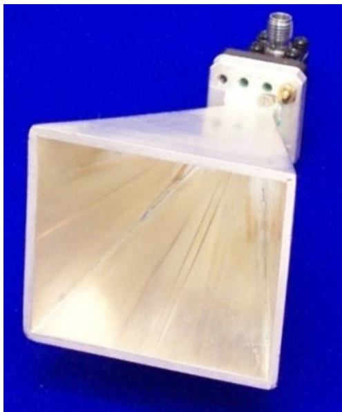
Fig. 5 Horn Antenna Developed by Conventional Method
