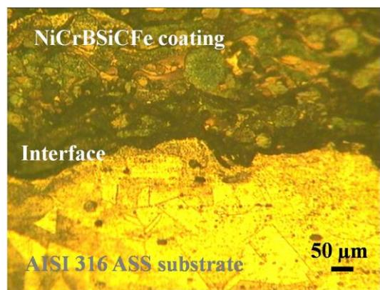
Fig. 5 Microstructure of NiCrBSiCFe Coating
