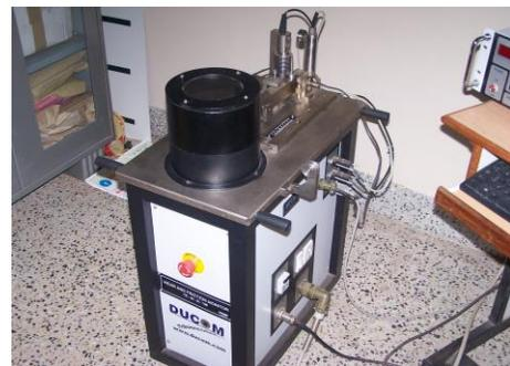
**Fig. 1 Experimental Setup for Wear Testing**
