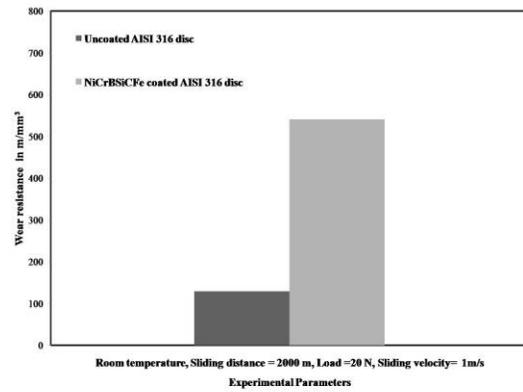
Fig. 8 Wear Resistance of Uncoated and NiCrBSiCFe Coated AISI 316 ASS
