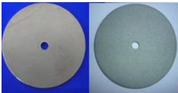
Fig. 4 Uncoated and NiCrBSiCFe Coated AISI 316 ASS
