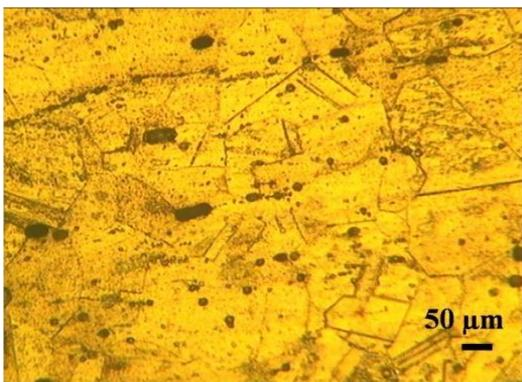
Fig. 3 Microstructure of AISI 316 ASS
