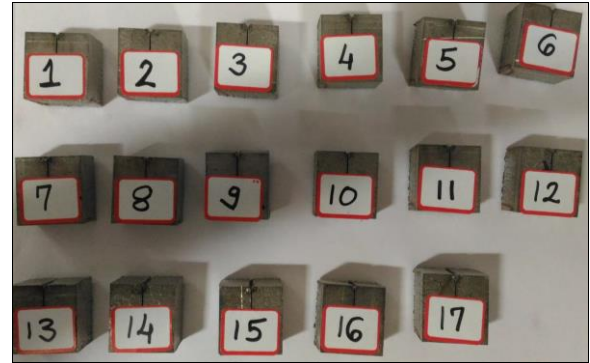
Fig. 3 Machined workpiece samples of AISI 304 material
