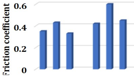
Fig. 3 Friction coefficients of selected plant-based, animal-based and hybrid brake pads
