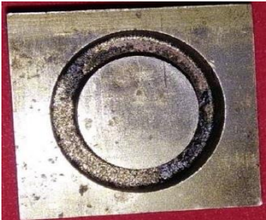
Fig. 3 Typical ram tensile test specimen of diffusion bonded ASS-Ti alloy joint
