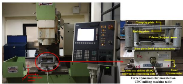
Fig. 3. Experimental setup for SPIF using dummy sheet
