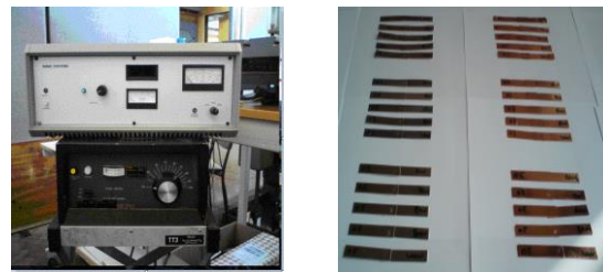
Figure 2 Setup of ultrasonic welding device and their accessories with generator, controller and sets of spot welded specimens
