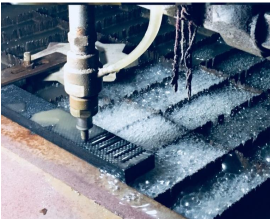
Fig. 1. Machining of carbon fibre vinyl ester composite by AWJM
