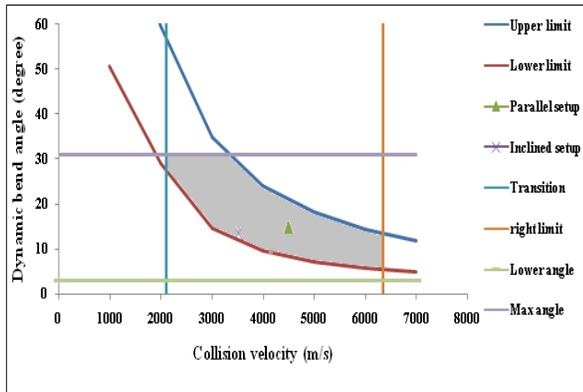
Fig. 2 Welding window for aluminium-magnesium explosive cladding
