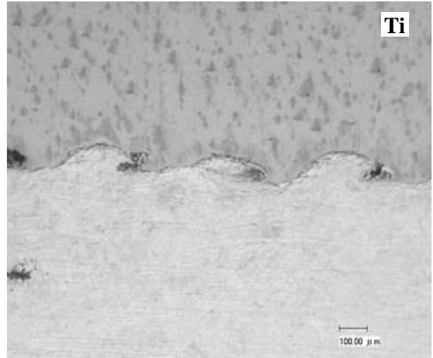
Fig. 4 Microstructure of Ti-Steel explosive clad
