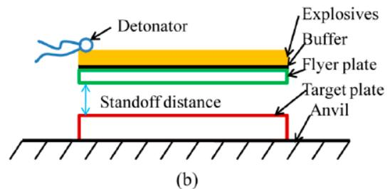
**Fig. 1 Explosive cladding configurations (a) Inclined (b) Parallel**
