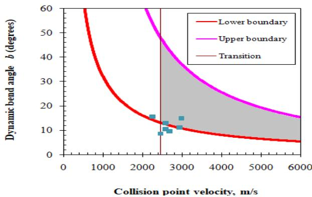
Fig. 3 Welding window for titanium-steel explosive cladding
