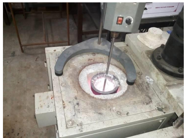
Fig. 1 Experimental setup for fabricating Al- \text{Al}_2\text{O}_3 and \text{B}_4\text{C} . Micro composites
