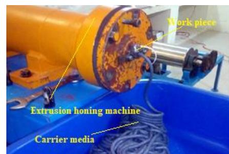
Fig. 2 Equipment for performing extrusion honing
