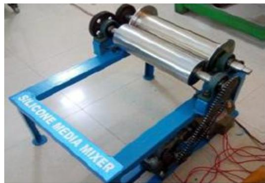
**Fig. 3 Carrier media mixing machine.**
