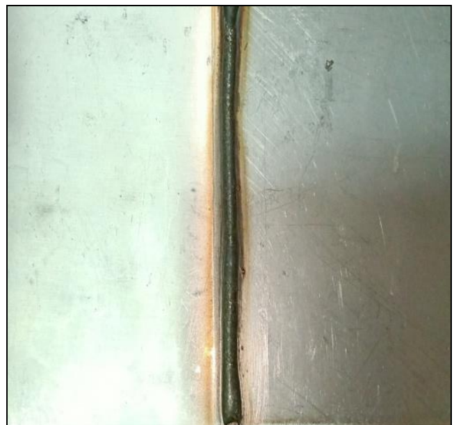
Fig. 4 Welded specimen automatic
