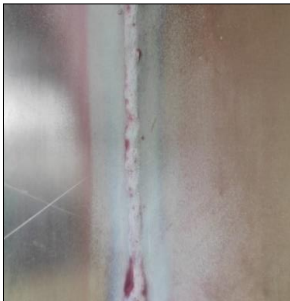
Fig. 6 LPT (developer solution)
