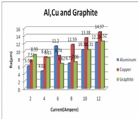
Fig. 4 Surface Roughness for all Electrodes
