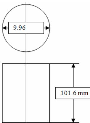
Fig. 1 Specifications of Electrode Used
