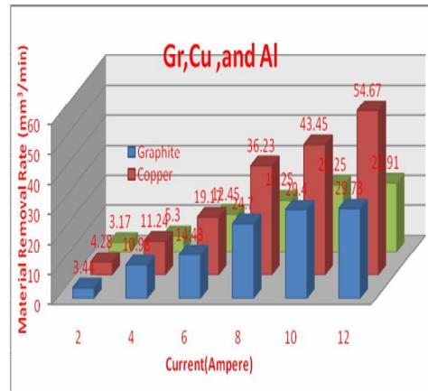
**Fig. 2 Material Removal Rates for all Electrodes**
