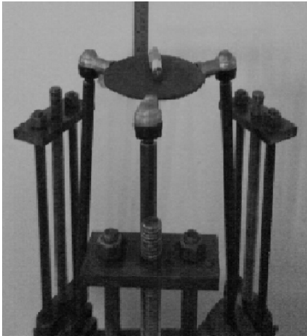
Fig. 3 Experimental Setup of Tripod Parallel Manipulator
