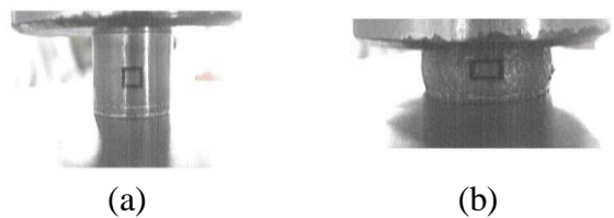
Fig. 9 Images of Grids Drawn at Equatorial Plane (a) Before Deformation and (b) After 50% Deformation
