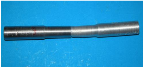
Fig. 9 Tensile Failure of the Friction Welded Component at Interface
