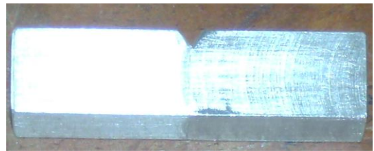
Fig. 1 Charpy Impact Test Sample of Dissimilar Metal
