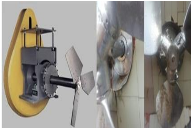
Fig. 2 Agitator and stuffing box
