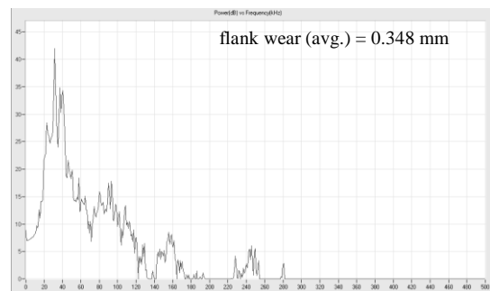
Fig. 6 Power Spectral Density Plot of AE Signal from Spindle Bearing 1 for Worn-out State of the Drill Bit
