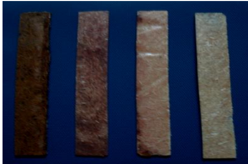
Fig.1 Physical Appearance of Short Roselle/Sisal Fiber Hybrid Polyester Composite
