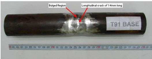
Fig.9 Visual inspection of failed base metal
