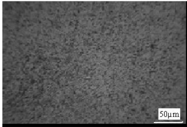
Fig.13 Microstructure of base in defect free region Higher hardness is due to the result of the tempered martensite and the carbides
