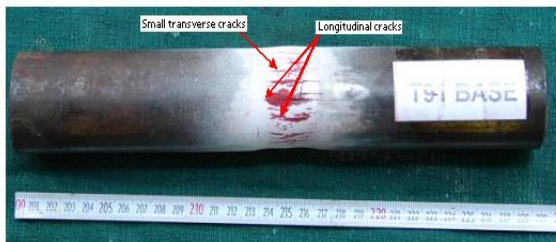
Fig.10 Liquid penetrant examination of failed base specimen
