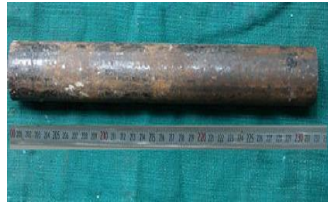
Fig.1 T-91 base tube before subjected to thermal fatigue
