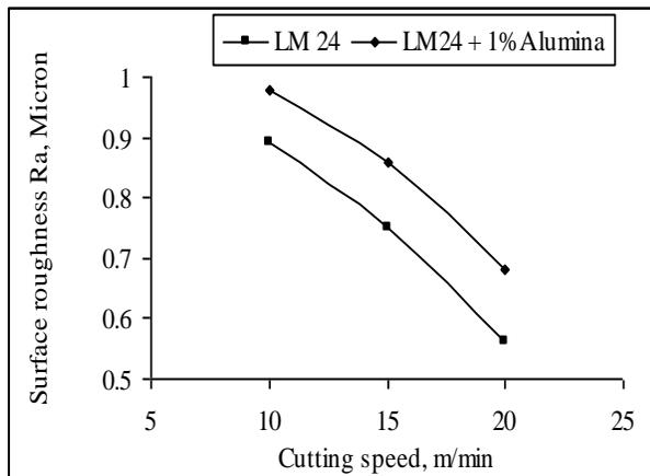
**Fig. 4** Surface roughness vs cutting speed at feed of 0.3 mm/rev
