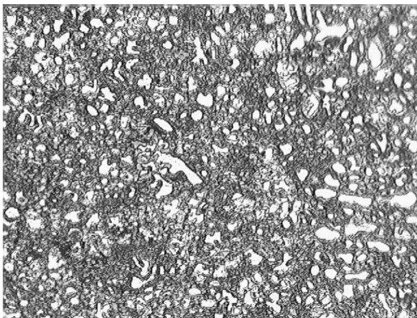
Fig. 1 The microstructure of the plain LM24 aluminum alloy
