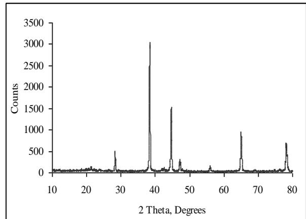
Fig. 2 XRD Pattern of the plain LM 24 aluminum alloy
