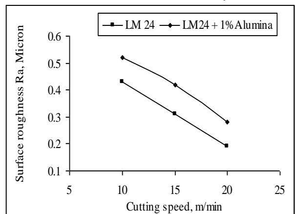
Fig. 3 Surface Roughness vs Cutting Speed at feed of 0.1 mm/rev
