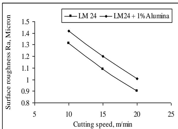
**Fig. 5** Surface roughness vs cutting speed at feed of 0.5 mm/rev
