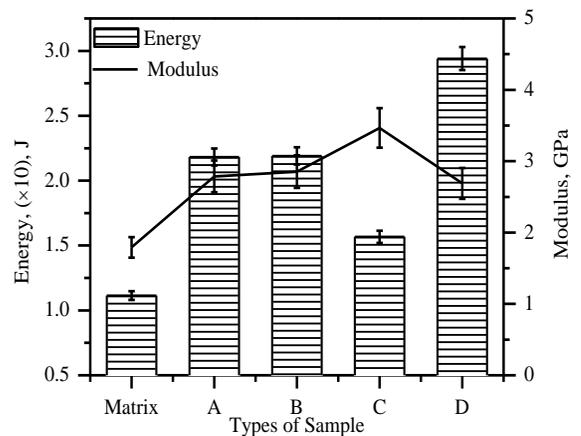
**Fig. 7 Comparison of Energy absorption and Young's modulus of different types of composite and the matrix**
