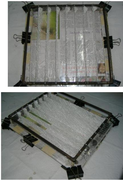
**Fig. 3 Strips of 5 mm width hung over the steel wire tied on the frame for Type D composite fabrication**
