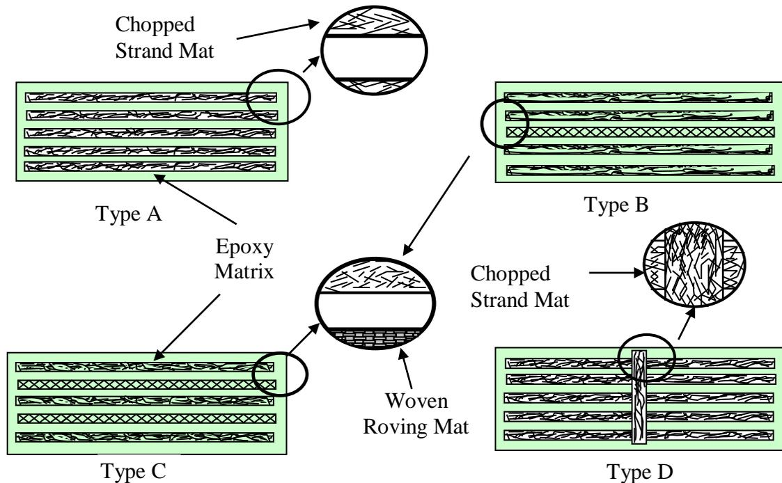
**Fig. 2 Schematic illustrations of glass fiber mats in different types of composite.**
