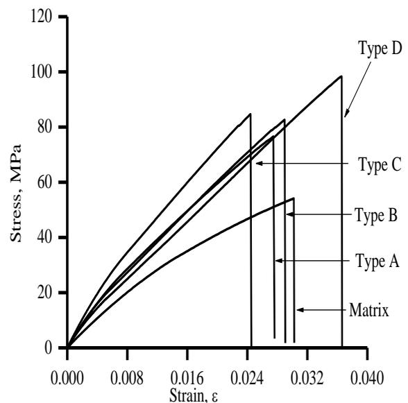
**Fig. 4 Stress-strain curves of different types of composite and matrix**
