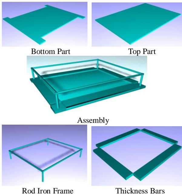
**Fig. 1 Components of die and their assembly**
