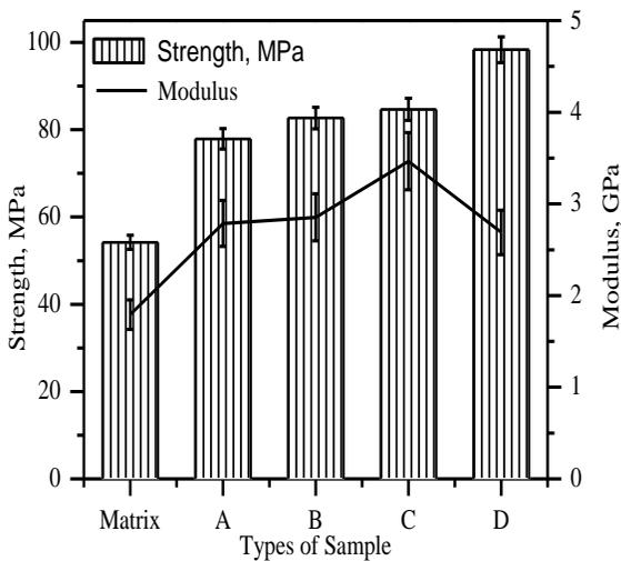
**Fig. 5 Comparison of strength and Young's modulus of different types of composite and the matrix**
