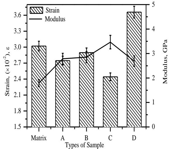
**Fig. 6 Comparison of strain and Young's modulus of different types of composite and the matrix**
