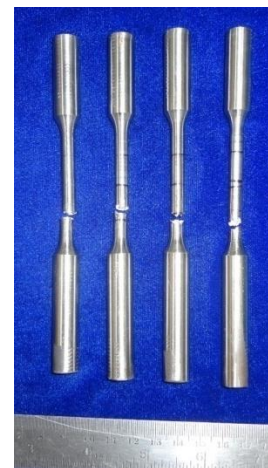
Fig. 2 Tensile Specimen after Tensile Test
