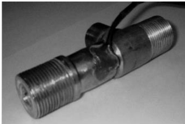
Figure 3 - Tube Specimen for Ratcheting Testing.
