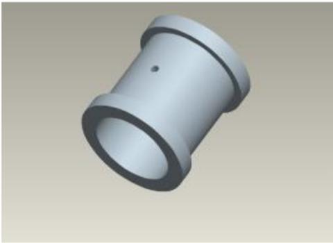
Fig. 5. Pressure vessel cylinder with circular hole
