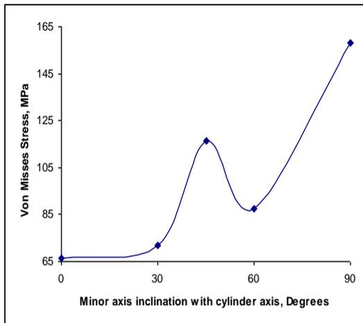
Fig. 13. Stress vs Inclination of the minor axis with cylinder axis.
