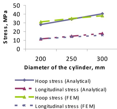
Fig. 3. Comparison of analytical and FEM result of Hoop & Longitudinal stresses in cylinders without hole
