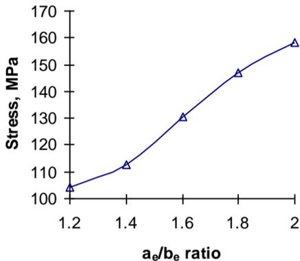
Fig. 9. Stress Vs  $a_e/b_e$  ratio for the major axis of an ellipse parallel to cylinder axis.
