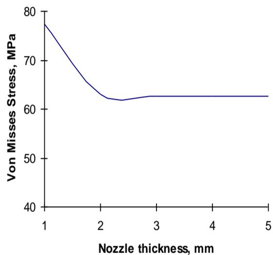
Fig. 18. Nozzle wall thickness, mm Vs Von misses stress, MPa.
