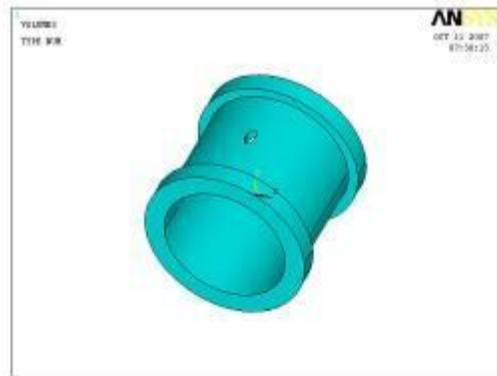
Fig. 8. Pressure vessel cylinder with elliptical hole major axis parallel to the cylinder axis.
