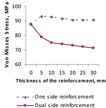
Fig. 14. Comparison of one sided reinforcement with both sided reinforcement.
