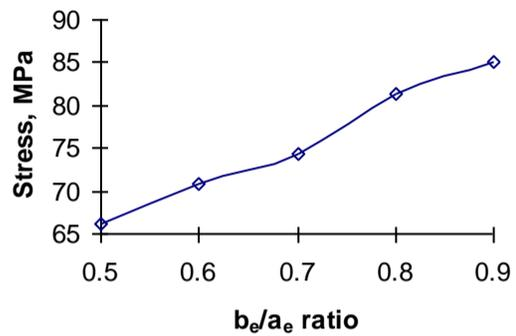
Fig. 11. Stress Vs  $b_e/a_e$  ratio for the major axis of an ellipse perpendicular to cylinder axis.
