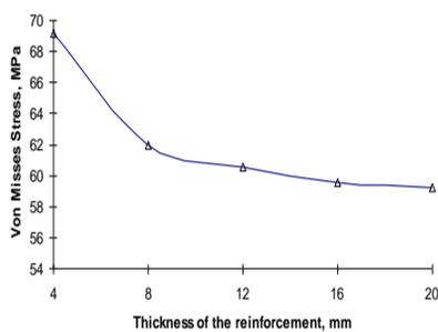
Fig. 16. Thickness of the reinforcement, mm Vs Von misses stress, MPa.
