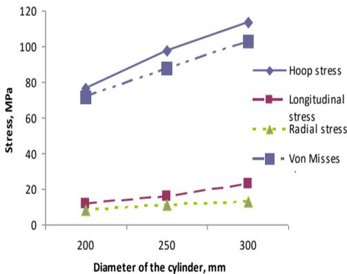
Fig. 6. Stress vs Diameter of the cylinder with circular hole.
