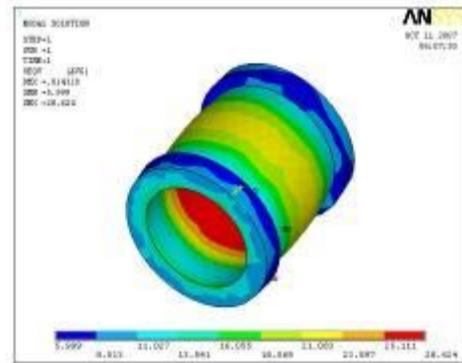
Fig. 2. Von Misses stress plot for 200mm diameter cylinder
