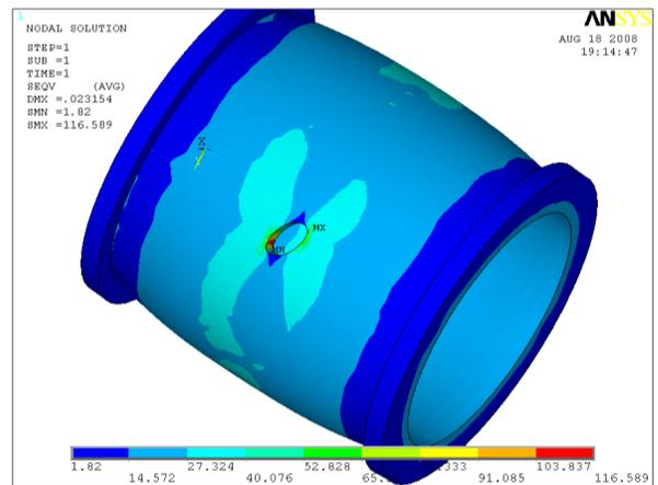
Fig. 12. Von misses stress plot for 250mm diameter cylinder with elliptical hole minor axis inclined at 45° to the cylinder axis
