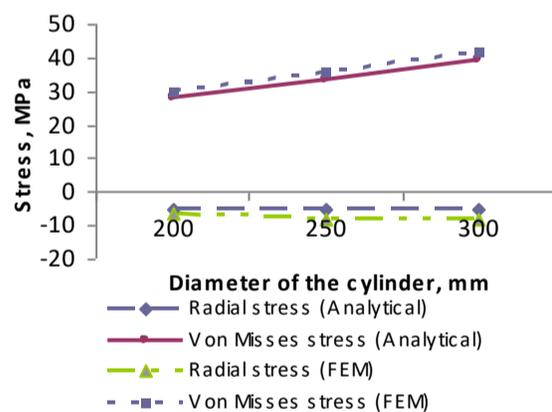
Fig. 4. Comparison of analytical and FEM result of Radial & Von Misses stresses in cylinders without hole
