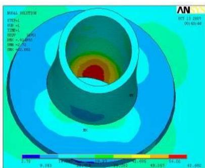
Fig. 17. Von Misses stresses plot for 250 mm diameter cylinder with 3 mm nozzle wall thickness.
