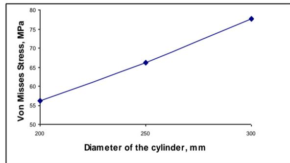
Fig. 7. Stress vs Diameter of the cylinder with elliptical hole major axis perpendicular to the cylinder axis
