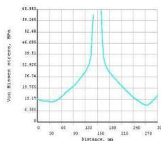
Fig. 15. Plot for Von misses stress Vs distance in 300mm height cylinder.
