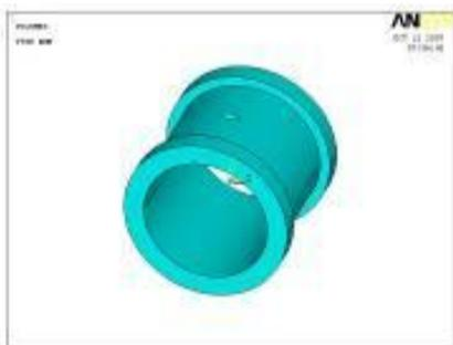
Fig. 10. Pressure vessel cylinder with elliptical hole major axis perpendicular to the cylinder axis.
