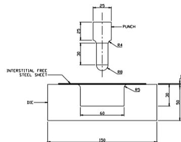
**Fig1. Schematic Diagram of the Experimental Setup**
