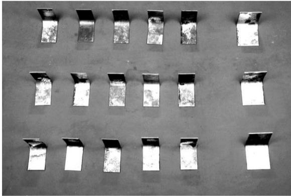
**Fig.2. Photographs of Deformed Samples of Different Widths(I<sup>st</sup> row-0°,II<sup>nd</sup> row-45°,III<sup>rd</sup> row-90°)**
