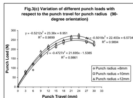
**Fig. 3 (a)-(c) have been drawn for different punch radius like 8mm, 10mm and 12mm between the punch load and punch travel provided punch velocity is kept constant.**
