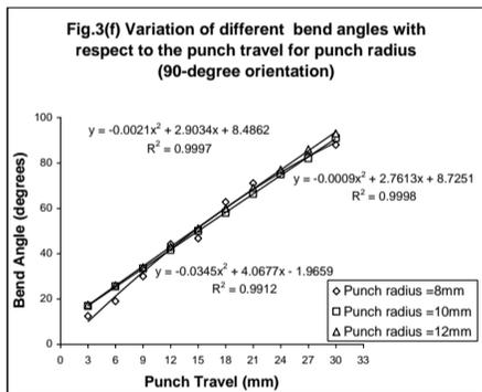
From the graphs Fig. 3 (d)-(f), it is noted that the punch travel versus bend angle under loading curves show a polynomial for different punch radii irrespective of orientations. The punch radius 12mm has make higher bend angle than 8mm punch radius. From these plots it is observed that the bend angle is dependent on punch radius.
