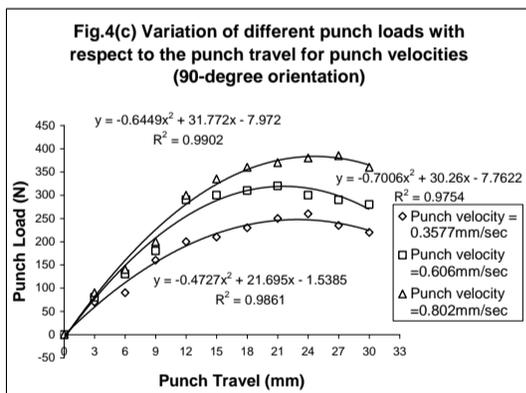
Fig. 4 (a)-(c) show that the punch load is higher for higher punch speeds ( $v=0.802\text{mm/s}$ ). This similar behavior has been observed for all orientations tested. For a particular speed, the punch load increases with
