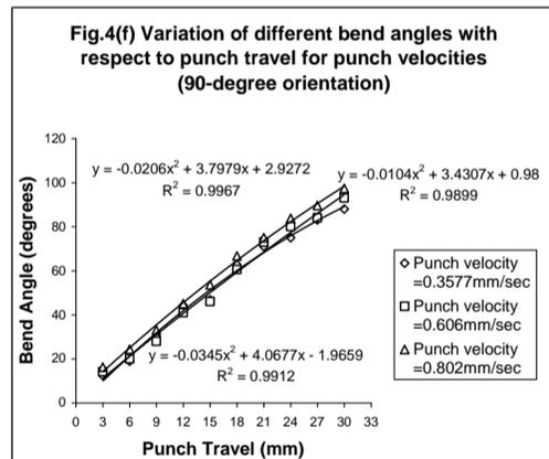
Fig. 4 (d)-(f) show the variation of different bend angles with respect to the punch travel for three orientations provided punch radius is kept constant. The punch travel versus bend angle graphs shows a
