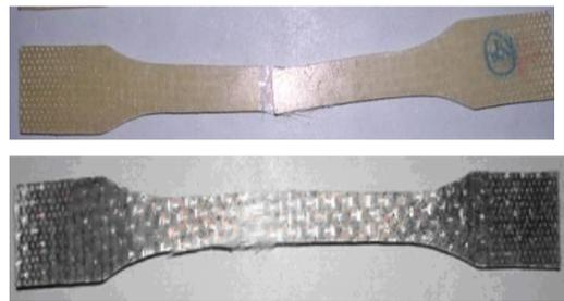
**Fig. 2 Fractured surface of G-P and SiC-G-P specimen**
