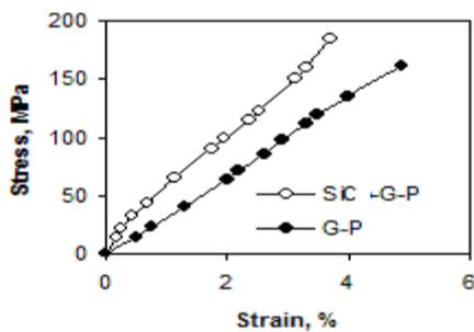
**Fig. 1 Stress vs. strain of G-P and SiC-G-P composites**
