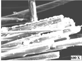
**Fig. 7b SEM picture of SiC-G-P composite showing broken fiber ends and matrix bonding**
