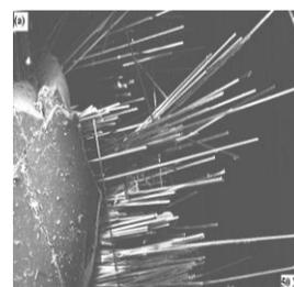
Fig. 7a SEM picture of SiC-G-P composite showing broken fiber ends and matrix bonding
