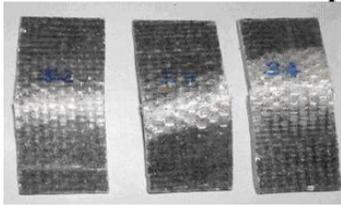
Fig. 5 Fractured surface of SiC-G-P flexure specimen
