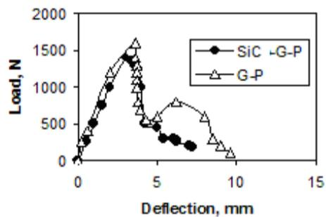
**Fig. 3 Load vs. deflection of G-P and SiC-G-P composites**
