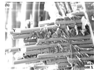
Fig. 6b SEM picture of G-P composite showing broken fiber ends and matrix bonding
