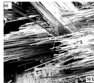
Fig. 6a SEM picture of G-P composite showing broken fiber ends and fiber-matrix debonding
