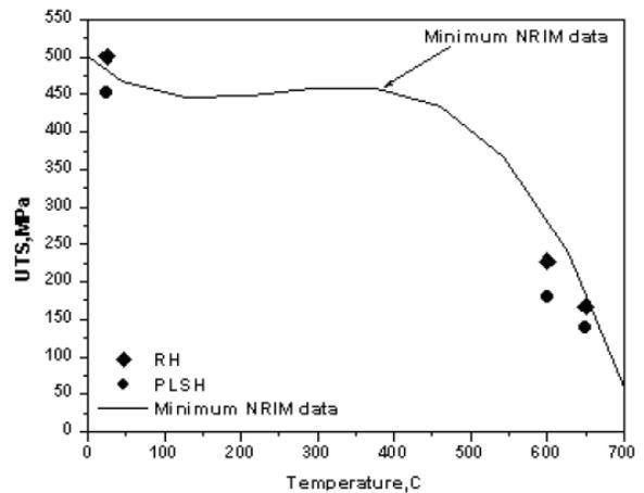
**Figure 13 - Temperature dependence of UTS of PLSH and RH tubes**
