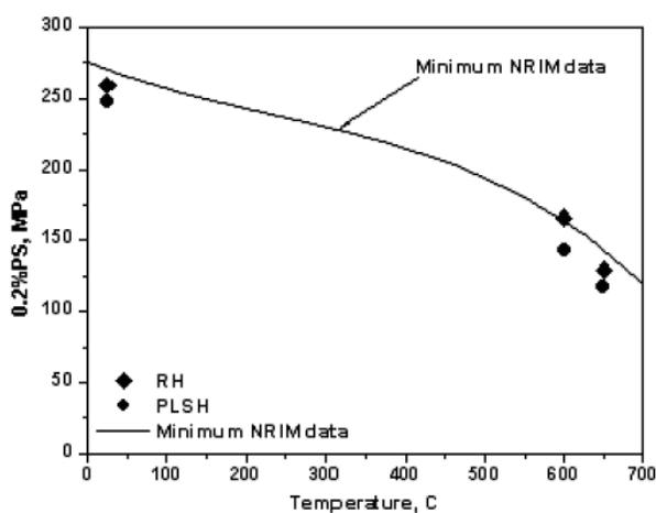
**Figure 12 -Temperaature dependence of 0.2% PS of PLSH and RH tubes**
