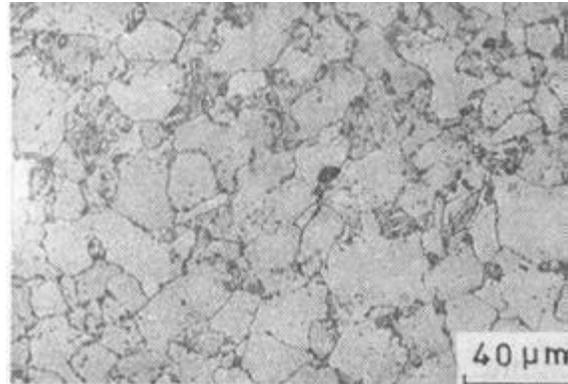
**Figure 8c** - Microstructures of a Failed tube showing freshly formed bainitic regions
