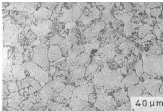
**Figure 8b**- Microstructures of Undamaged tube consisting of ferrite and tempered bainite
