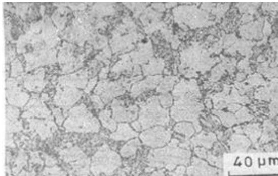
**Figure 8a** - Microstructures of Virgin tube
