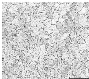
Figure 3 -. Micro structure of FSH tube
