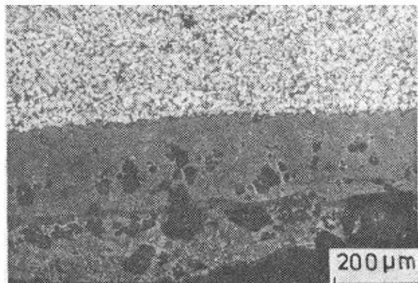
**Figure 9a** - 0.25 mm oxide scale at inner surface of failed tube
