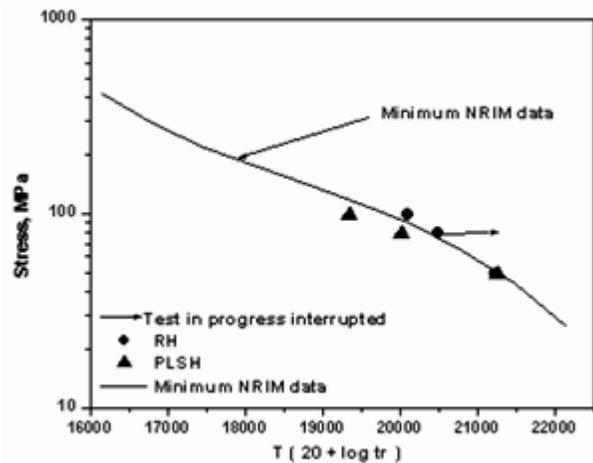
**Figure 14 - Stress Vs LMP plot of platen super heater and reheater tubes**
