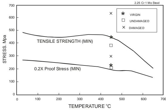
**Figure 7** - Tensile Properties of virgin, undamaged failed and failed final super heater tube of 500 MW Boiler
