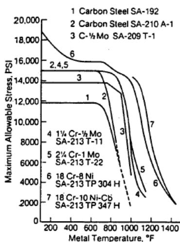
Figure 1 - Allowable stress for several grades of steel as a function of steel
