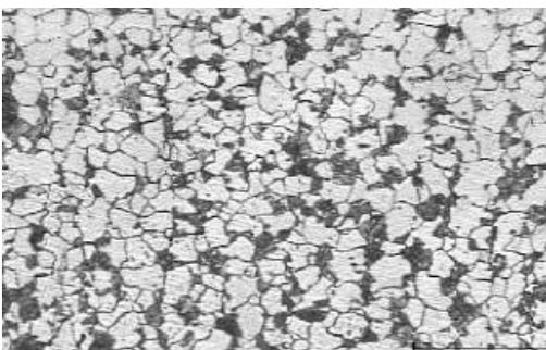
Figure 5 - Microstructure of LTSH tube
