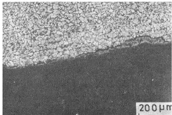
**Figure 9b** - Insignificant oxide scale at inner surface of the undamaged tube
