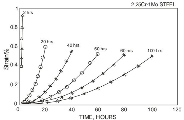
**Figure 11**- Predicted creep strain corresponding to time-temperature profile shown in Figure.10.
