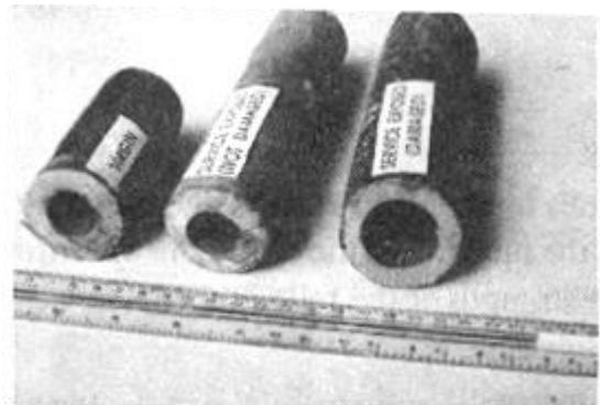
Figure 6 - Virgin, undamaged and failed super heater tube of 500 MW boiler
