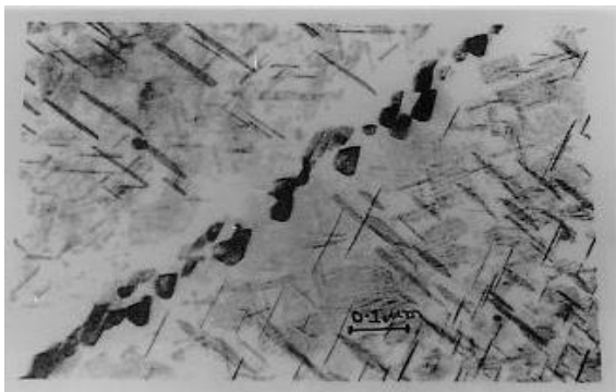
Figure 5 -Grain Boundary Microstructure of the Al-4% Cu-0.3% Mg-0.4% Ag
