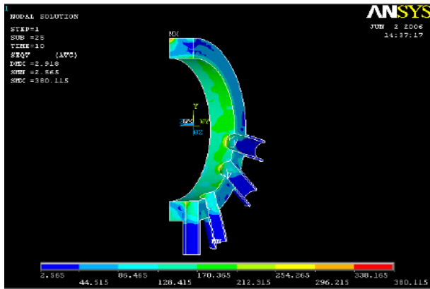
Figure 3 .- Von-Mises equivalent stress from the finite element analysis
